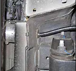
Installed Fuel fill With backup sensor. Torque six hex bolts to 35-40in lb.
