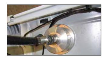
When feeding the HP hose into the car follow the OEM fuel fill hose. Use two P-clamps to secure it to the car and zip tie as needed to keep the HP line from moving around.
